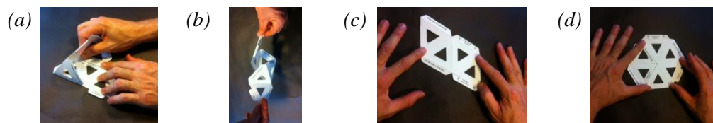
Figure 3: Folding patterns of building unit(s): (a) tetrahedral folding; (b) spiraling folding governed by the attraction mode of the two poles of the chained helix-like ribbon; (c) folding into a parallelogram building unit; (d) folding into a hexagon building unit
